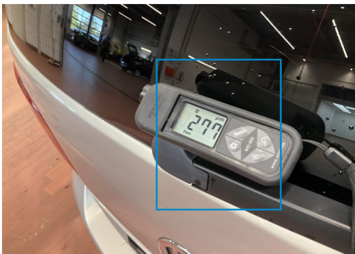
1. Tailgate Paint / Poor Previous Repair -
