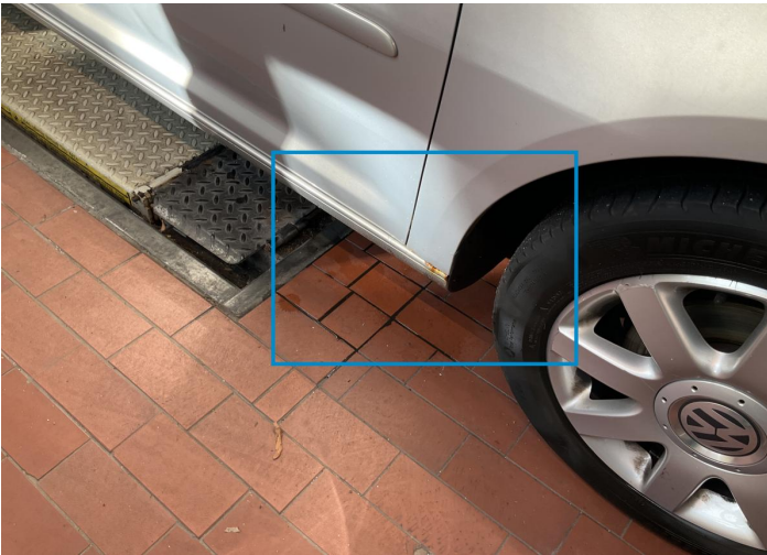
13. Rocker Panel / Center Right Paint / Corrosion -
