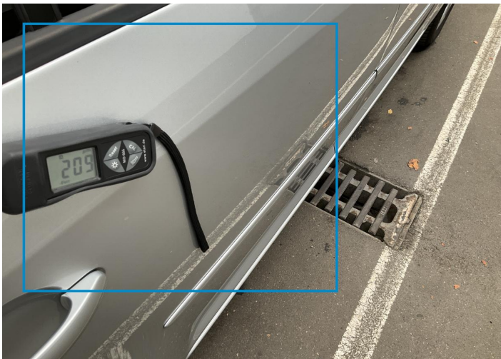
8. Door / Back Right Paint / Poor Previous Repair -
