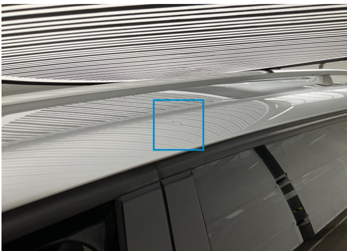
26. Pillar / Back Left Bodywork / Dent / Dent -
