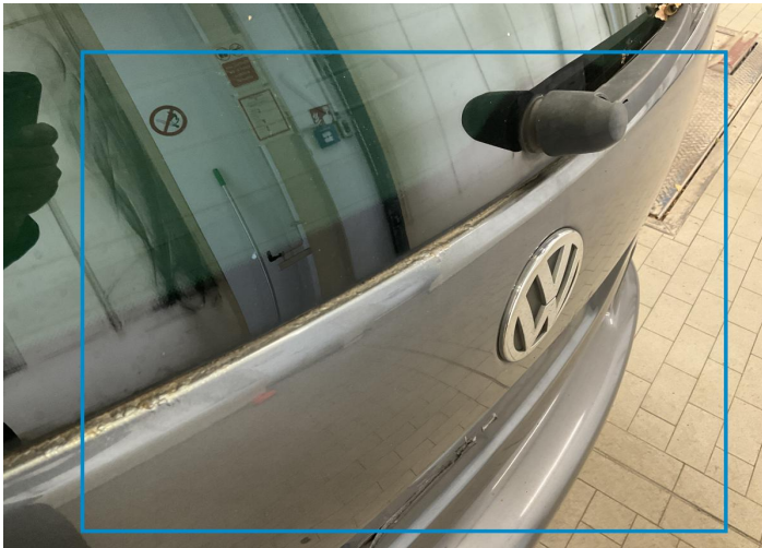
9. Tailgate Paint / Corrosion -
