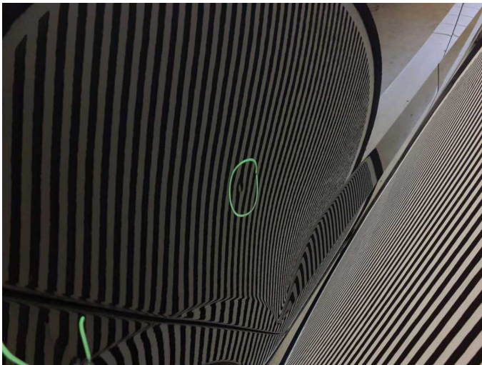
Damage 5: Door - rear right side: Door (1 Delle+Knick) - dent(s) - Smart repair
