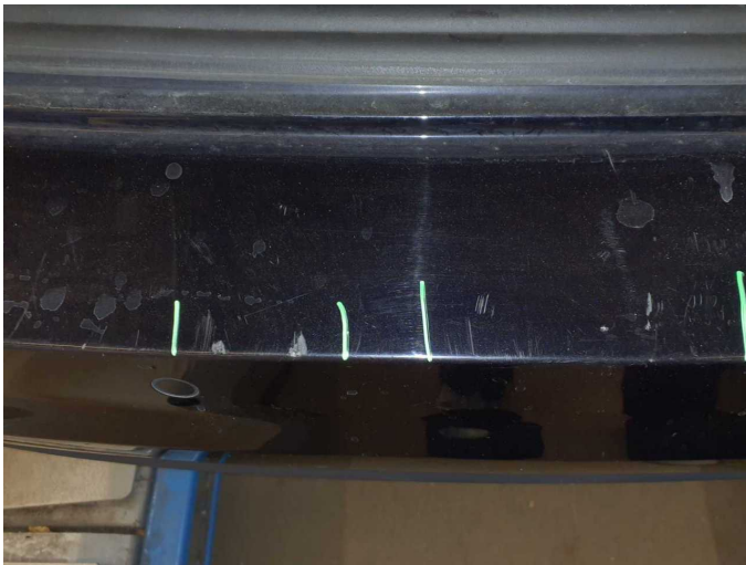
Damage 8: Rear bumper: Rear bumper - Scratch(es) - Paint
