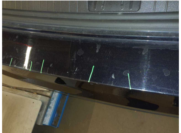
Damage 8: Rear bumper: Rear bumper - Scratch(es) - Paint
