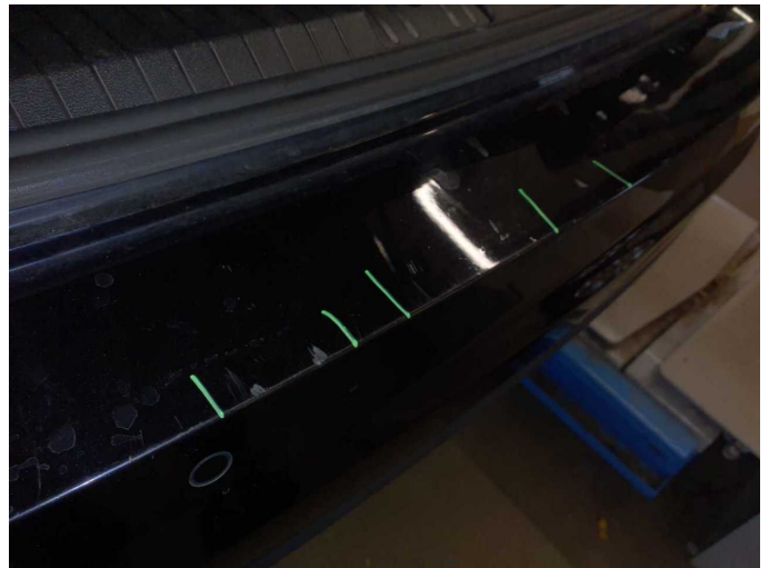
Damage 8: Rear bumper: Rear bumper - Scratch(es) - Paint
