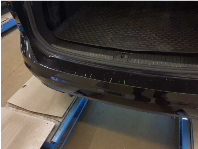
Damage 8: Rear bumper: Rear bumper - Scratch(es) - Paint
