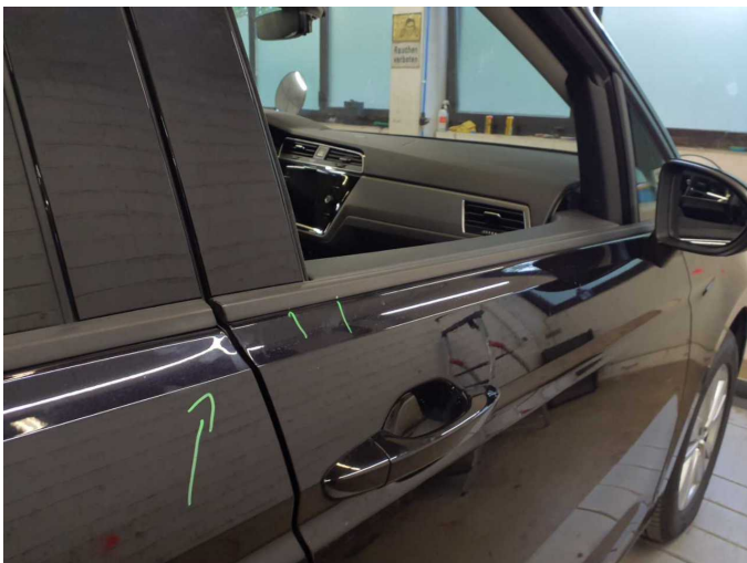
Wear and tear 2: Door - front right side: Door - dent(s) - Smart repair
