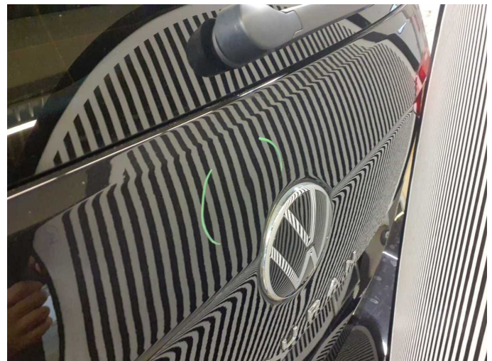
Damage 1: Boot lid / rear door: Boot lid (1) - dent(s) - Smart repair
