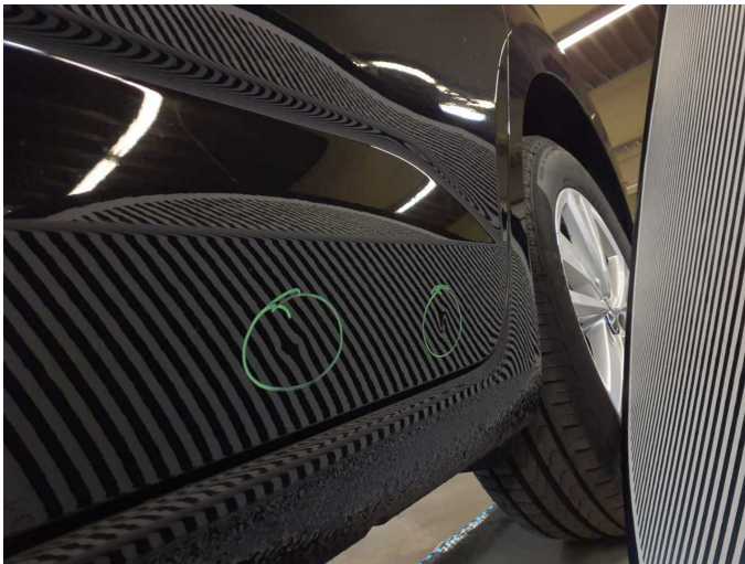
Damage 2: Door - rear left side: Door (2) - dent(s) - Smart repair
