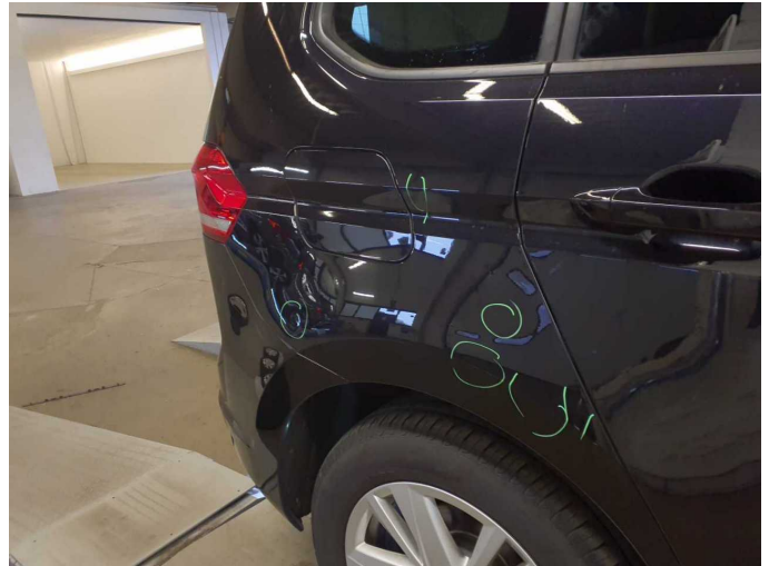
Damage 6: Side panel - rear right side: Side panel (6) - dent(s) - Smart repair
