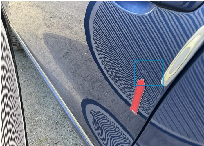
5. Door / Front Left Bodywork / Dent / Dent -
