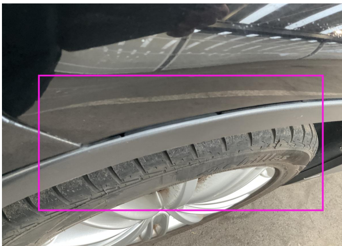
15. Wing Stick / Front Left Bodywork / Breakage / Crack -
