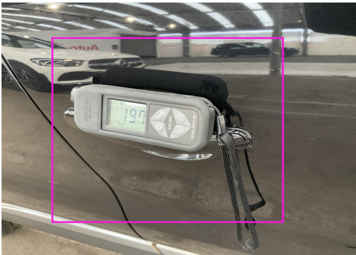
7. Door / Front Right Paint / Poor Previous Repair -
