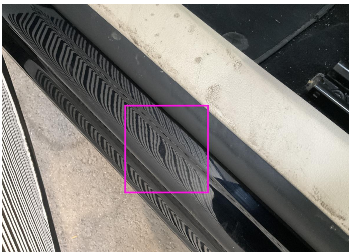
18. Rocker Panel / Center Left Bodywork / Dent / Dent -
