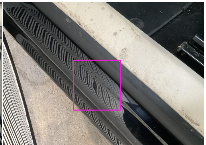
18. Rocker Panel / Center Left Bodywork / Dent / Dent -
