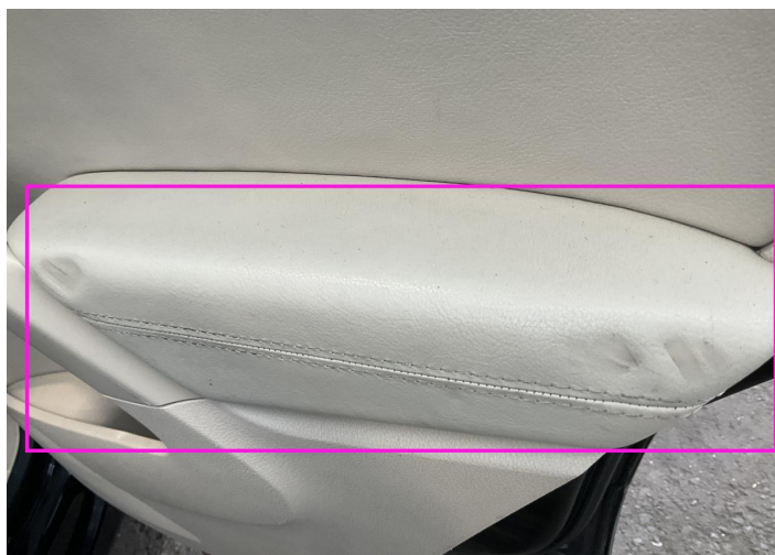
29. Panel Filling / Back Right Interior / Broken -
