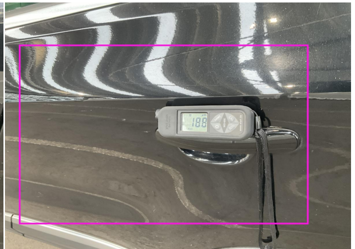
4. Door / Back Left Paint / Poor Previous Repair -
