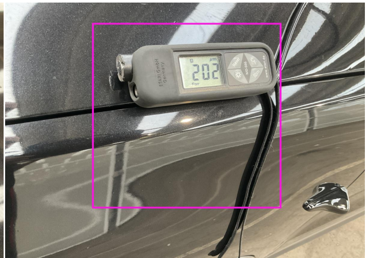
2. Wing Repeater / Left Paint / Poor Previous Repair -
