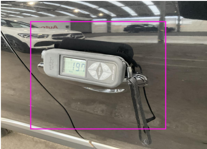
7. Door / Front Right Paint / Poor Previous Repair -
