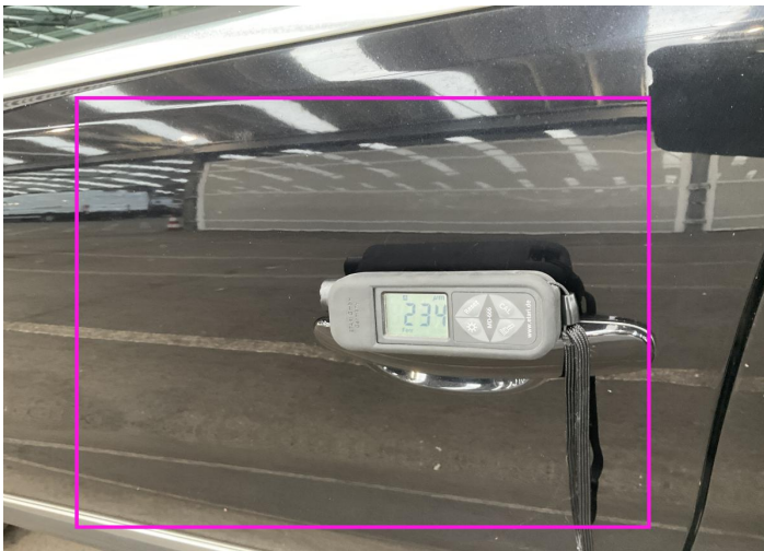
3. Door / Front Left Paint / Poor Previous Repair -
