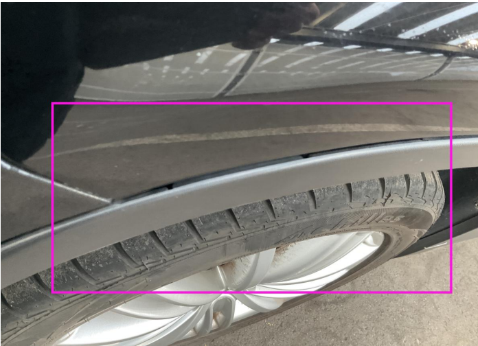
15. Wing Stick / Front Left Bodywork / Breakage / Crack -
