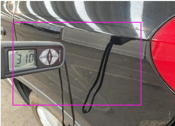
5. Fender / Back Left Paint / Poor Previous Repair -
