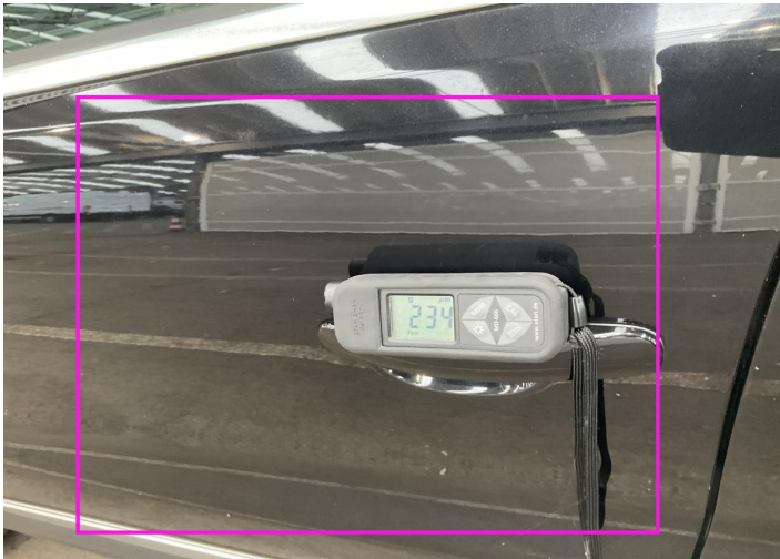
3. Door / Front Left Paint / Poor Previous Repair -
