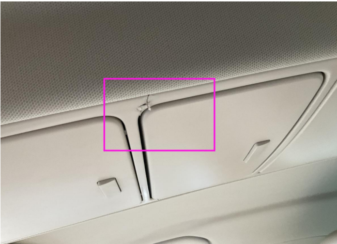
33. Roof Upholstery Interior / Broken -
