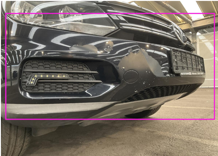
9. Bumper / Front Paint / Poor Previous Repair -
