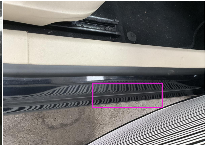
32. Rocker Panel / Center Right Bodywork / Dent / Dent -
