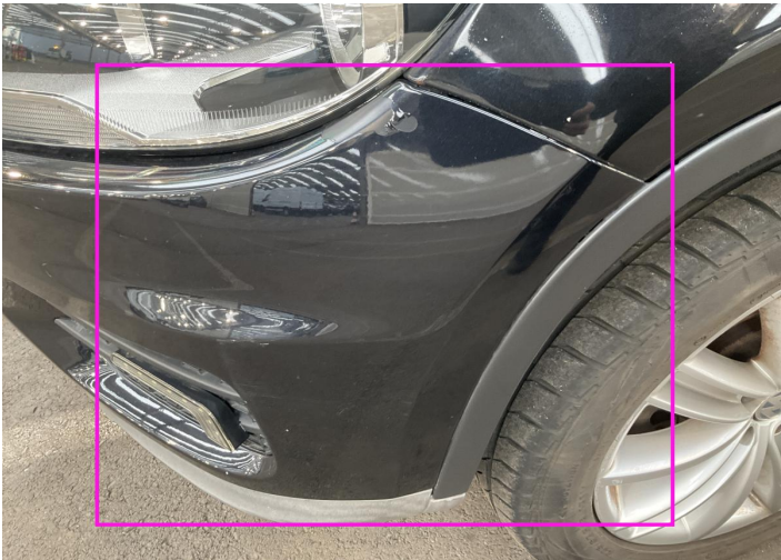
10. Corner Bumper / Front Left Bodywork / Breakage / Crack -
