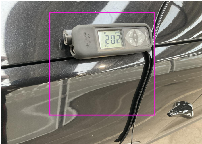
2. Wing Repeater / Left Paint / Poor Previous Repair -
