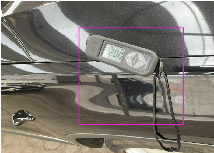
6. Fender / Front Right Paint / Poor Previous Repair -
