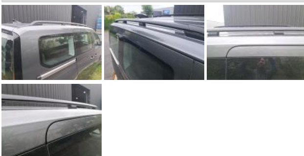
Roof pillar R, Scratch(es), Acceptable
