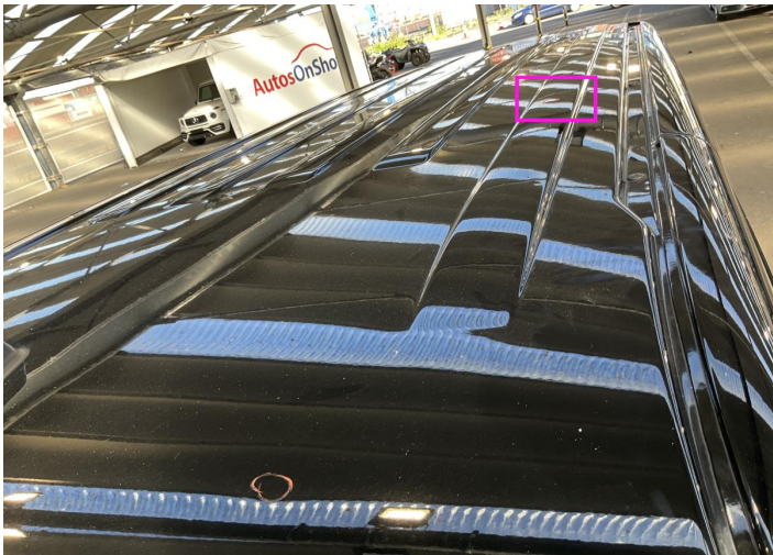
11. Roof Bodywork / Dent / Dent -
