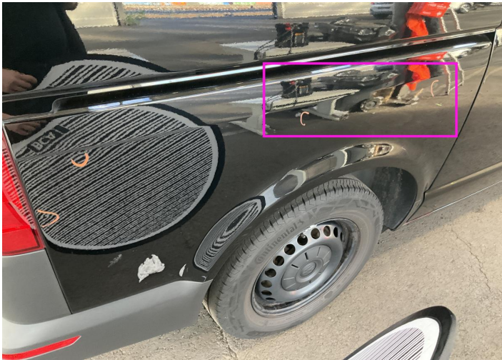
7. Side Panel / Back Right Bodywork / Dent / Dent -
