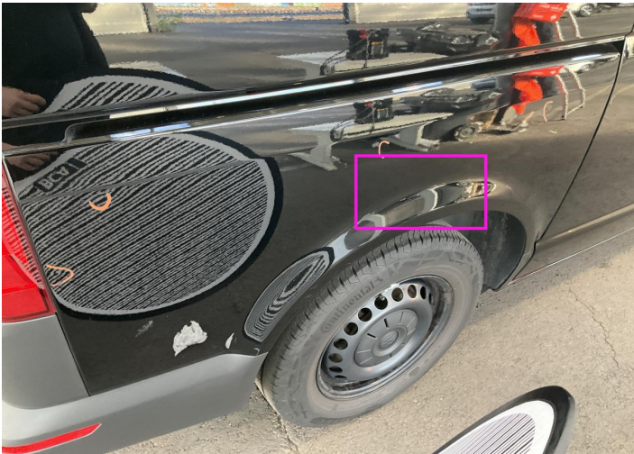
8. Side Panel / Back Right Paint / Scratch / Scuff -
