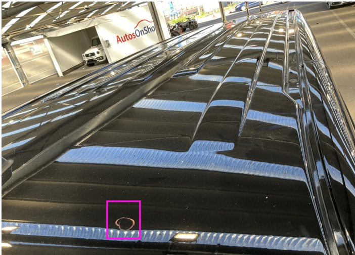
10. Roof Bodywork / Dent / Dent -
