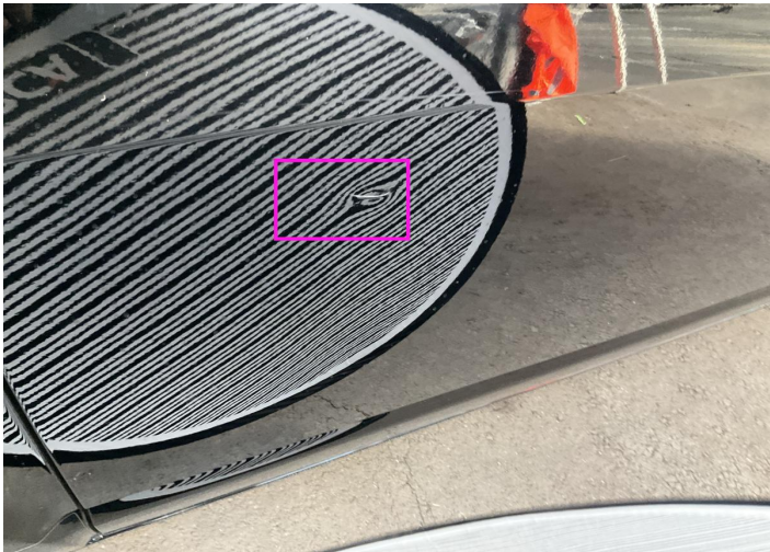
9. Door / Back Right Bodywork / Dent / Dent -
