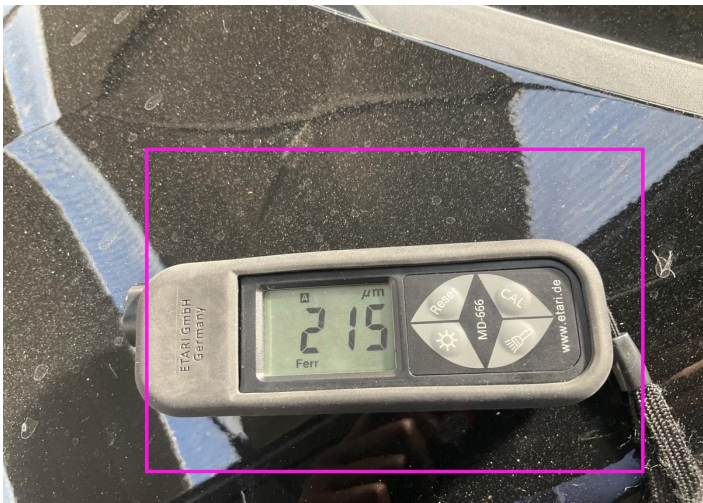
1. Fender / Front Left Paint / Poor Previous Repair -
