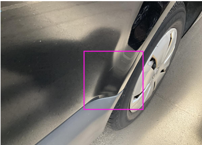
7. Side Panel / Back Right Paint / Scratch / Scuff -
