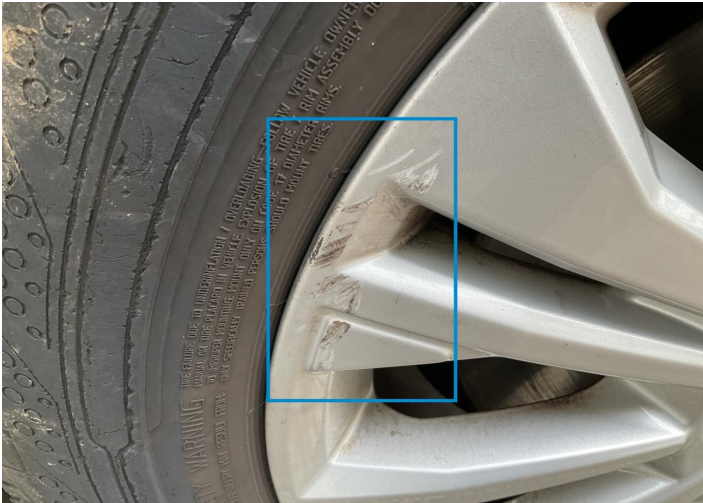
12. Rim / Front Right Out of Bodywork / Scratch -
