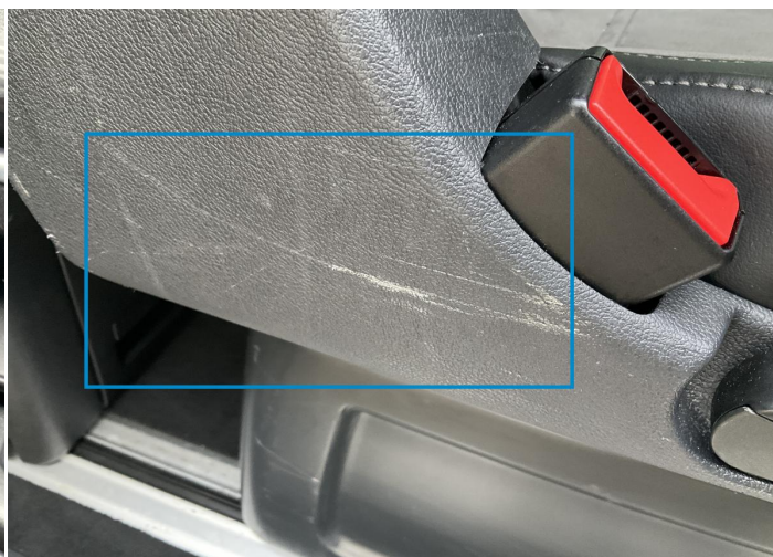
2. Seat / Back Right Interior / Scratched -
