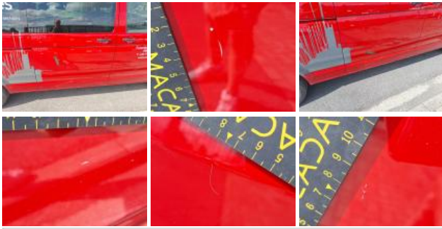
Door FR, Scratch(es), Repair and paint (complete)
