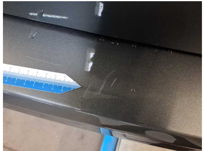
Damage 5: Rear bumper: Rear bumper - Scratch(es) - Paint
