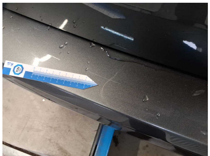
Damage 5: Rear bumper: Rear bumper - Scratch(es) - Paint
