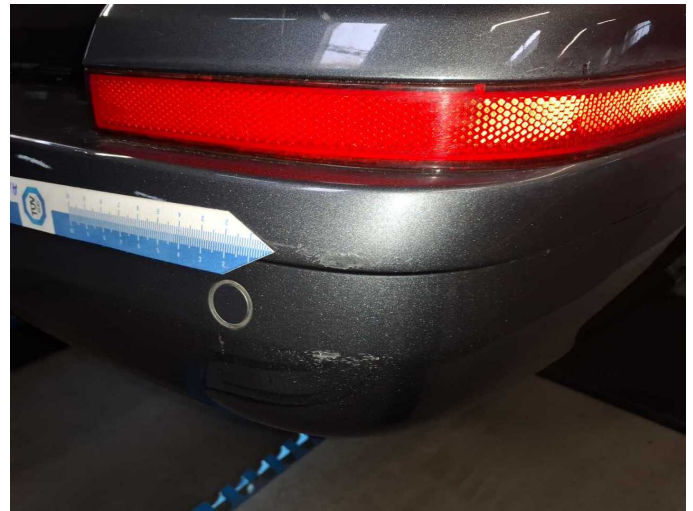
Damage 5: Rear bumper: Rear bumper - Scratch(es) - Paint
