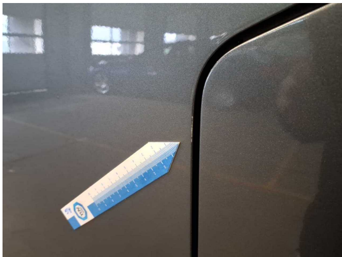
Wear and tear 1: Door - front left side: Door edge - Scratch(es) - Smart repair
