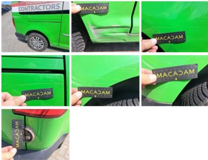
Door RR, Dent(s) and scratch(es), Spot repair
