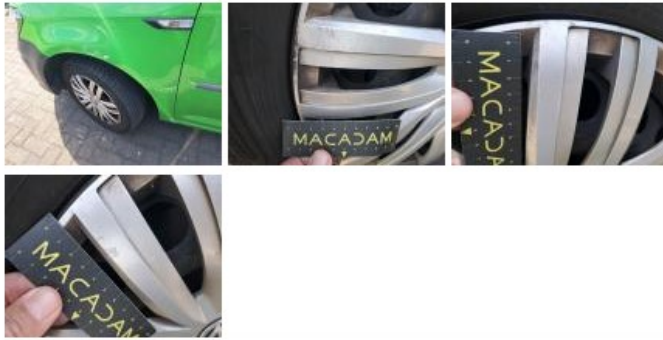
Wing FL, Dent(s), Paintless dent repair
