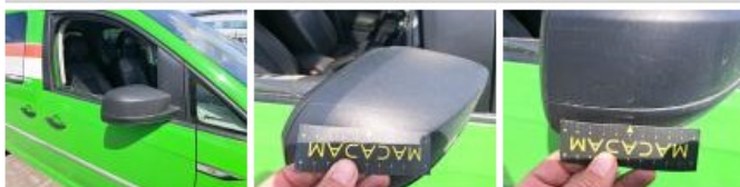
Wing FR, Dent(s), Repair and paint (complete)
