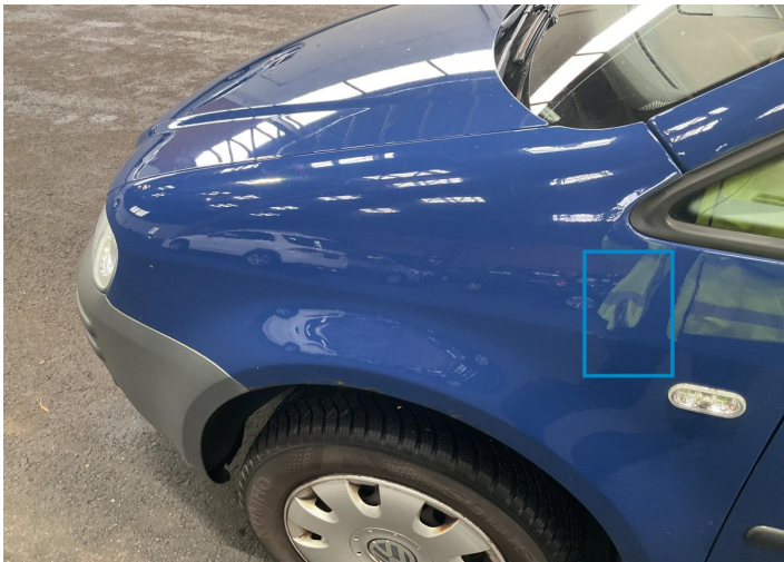
6. Fender / Front Left Bodywork / Dent / Dent -
