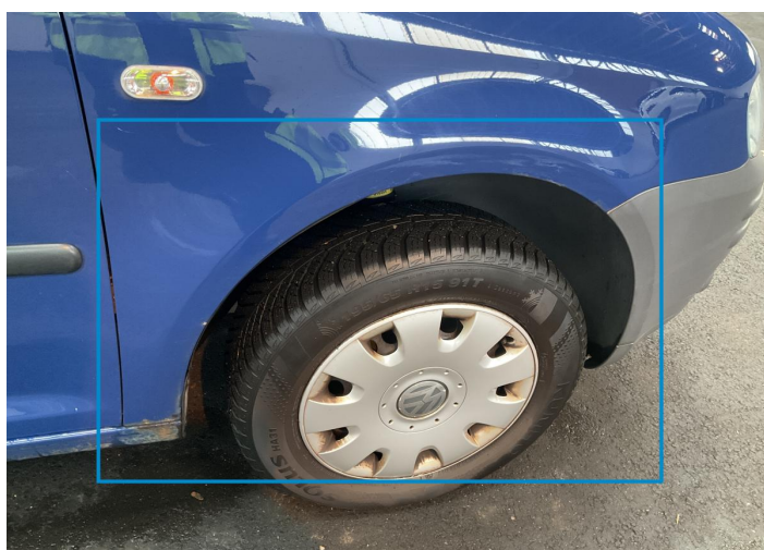
29. Fender / Front Right Paint / Corrosion -
