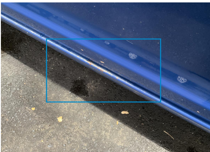
12. Rocker Panel / Center Left Paint / Corrosion -
