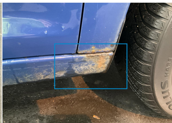
30. Rocker Panel / Center Right Paint / Corrosion -
