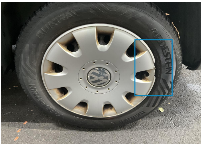
33. Hubcap / Back Left Out of Bodywork / Breakage -
