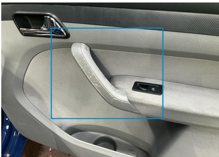
31. Panel Filling / Front Right Interior / Scratched -
