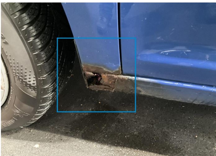
8. Fender / Front Left Paint / Corrosion -
