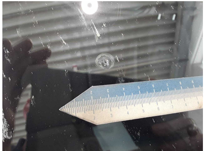
Damage 2: Vehicle glazing: Windscreen - Damaged - Replace
