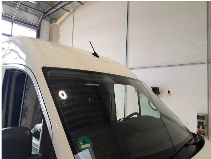
Damage 2: Vehicle glazing: Windscreen - Damaged - Replace
