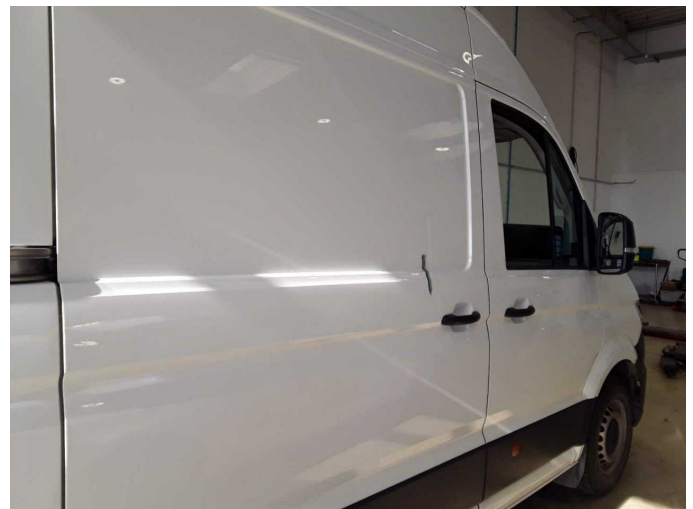
Damage 1: Sliding door, right: Sliding door - dent(s) - Smart repair
