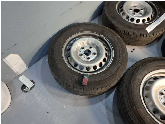
Damage 7: 2nd wheel set: 3 tyres (Profil kleiner 4mm) - Replace
