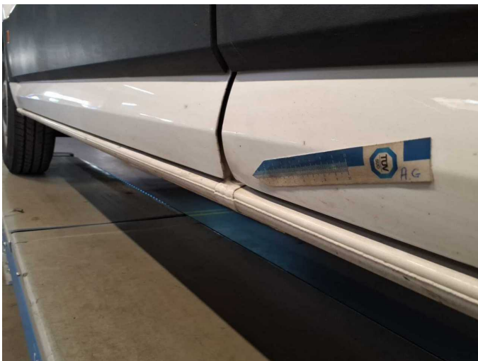
Damage 5: Door - front right side: Door - Deformed - Smart repair
