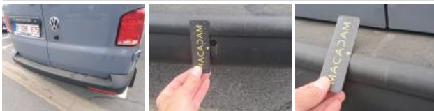
Boot door panel RR, Scratch(es), Spot repair
