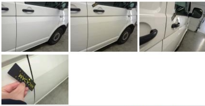
Wing FR, Scratch(es), Repair and paint (complete)
