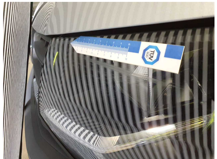
Damage 9: Headlight: Headlight - left side - Scratched - Replace
