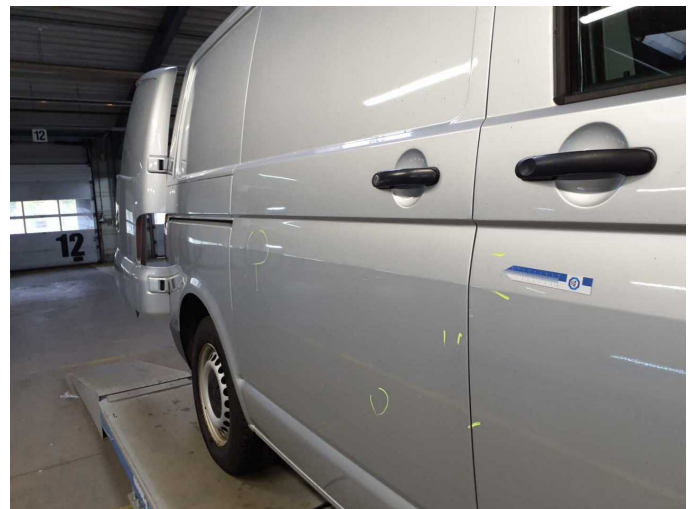
Damage 6: Door - front right side: Door - Scratched - Smart repair
