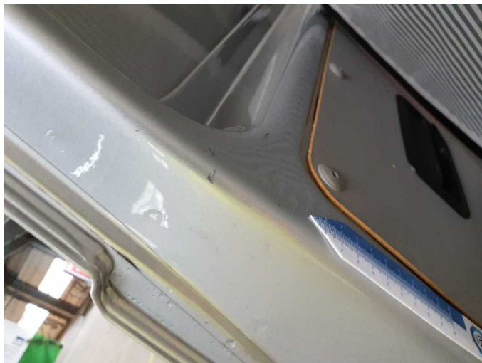
Damage 13: Boot lid / rear door: Rear door - left side (Kratzer) - Dent / paintcoat damage - Repair and paint
