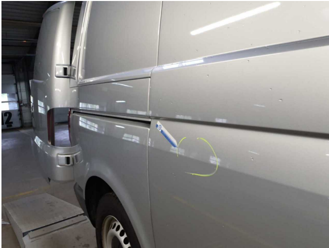
Damage 11: Sliding door, right: Sliding door (Dellen) - Scratched - Repair and paint
