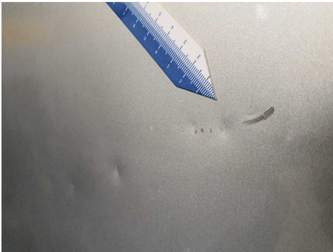
Damage 12: Boot lid / rear door: Rear door - right side (Kratzer) - Deformed - Repair and paint
