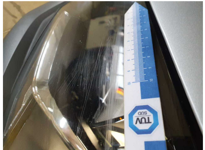
Damage 9: Headlight: Headlight - left side - Scratched - Replace
