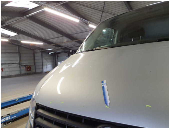
Damage 10: Bonnet: Bonnet (Steinschlag) - Corrosion - Repair and paint
