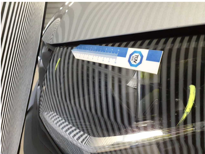
Damage 9: Headlight: Headlight - left side - Scratched - Replace
