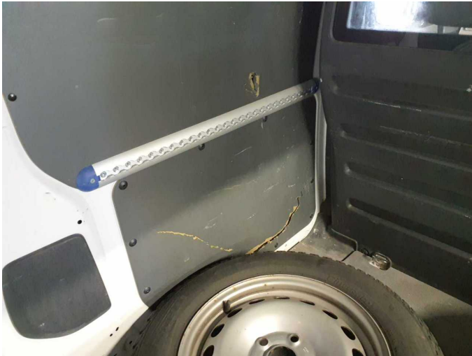
Damage 5: Trim / covers: Cargo area - lining -left side - Broken / torn - Replace
