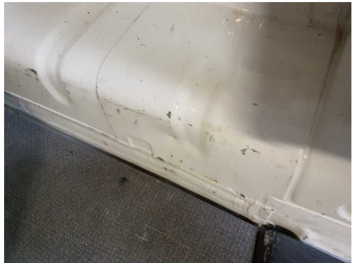
Damage 7: Interior: Interior (SEITENTEIL H I R) - Scratched - Smart repair
