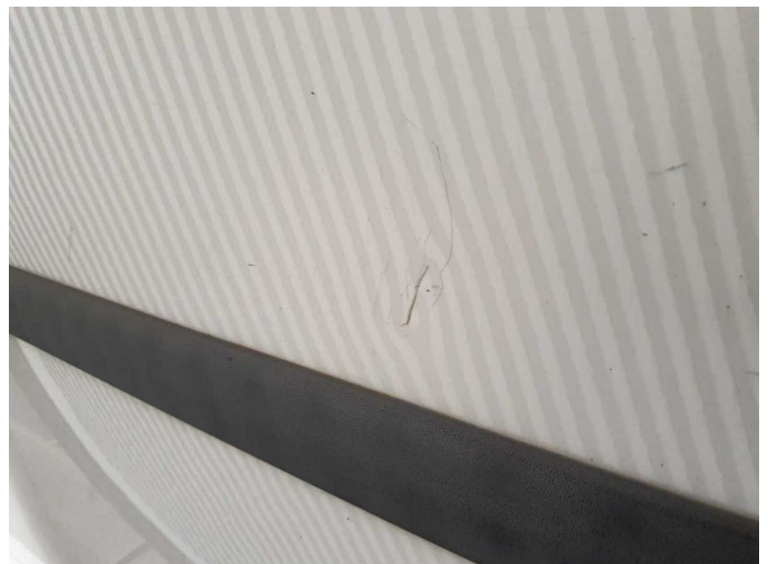
Damage 16: Sliding door, right: Sliding door (Kratzer) - Dent / paintcoat damage - Repair and paint
