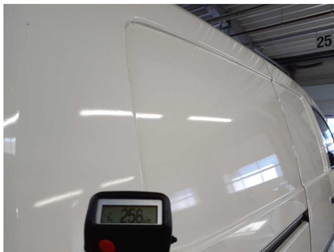
Repainting 1: Side panel - rear right side
