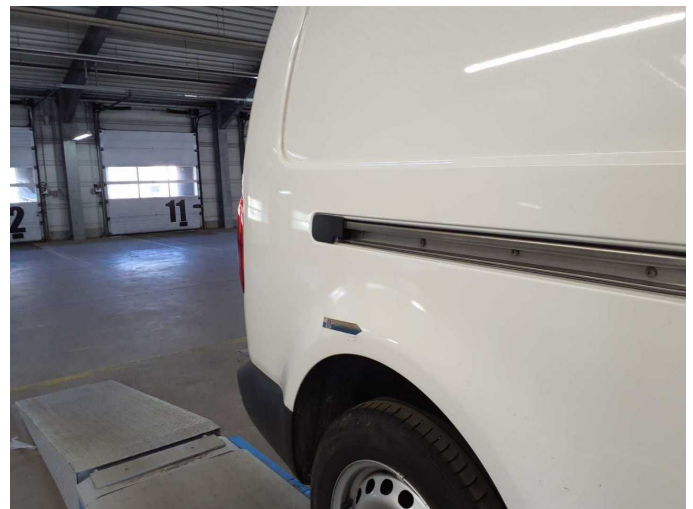
Damage 11: Side panel - rear right side: Side panel - Scratched - Smart repair
