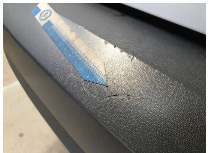
Damage 12: Rear bumper: Rear bumper - Scratched - Loss in value
