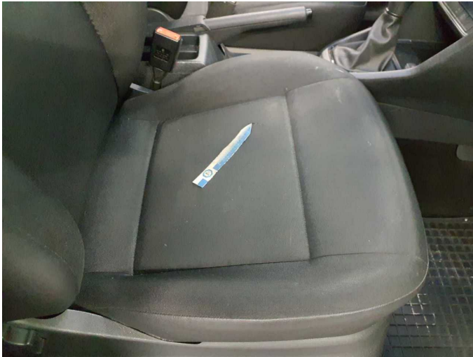
Damage 15: Seat - front: Seat cover - right side - Holes - Replace
