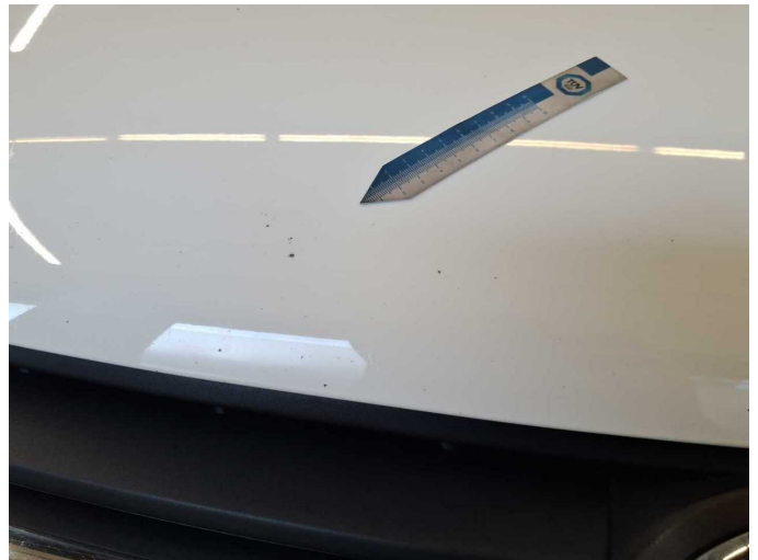
Damage 9: Bonnet: Bonnet - Stone chips - Paint
