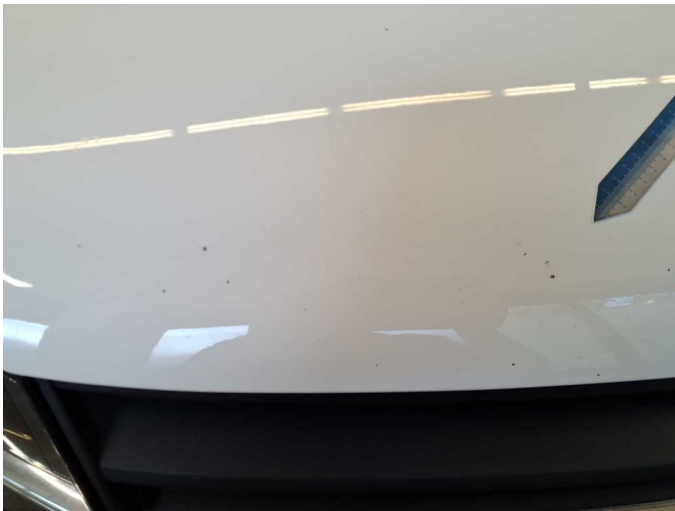
Damage 9: Bonnet: Bonnet - Stone chips - Paint
