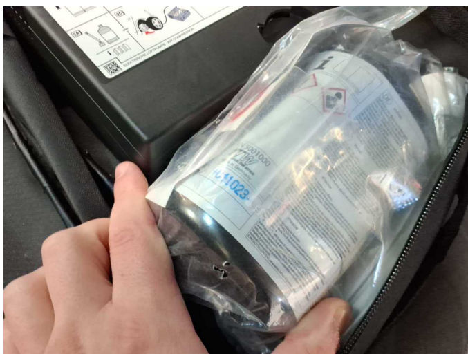
Damage 1: Equipment: Tirefit filler - Expired - Replace
