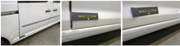
Door FR, Dent(s), Repair and paint (complete)
