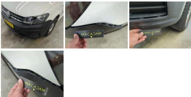
Bumper grille FR, Deformed / Strained, Replace
