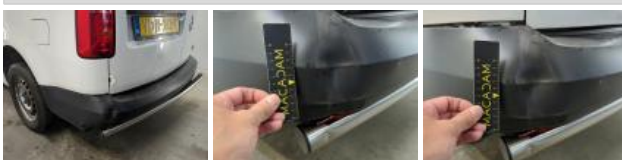
Reflector, Broken, Replace
