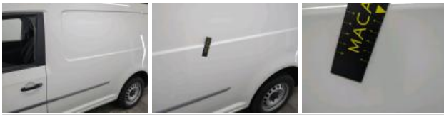
Outer sill L, Scratch(es), Repair and paint (complete)
