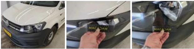
Wing FR, Dent(s), Repair and paint (complete)
