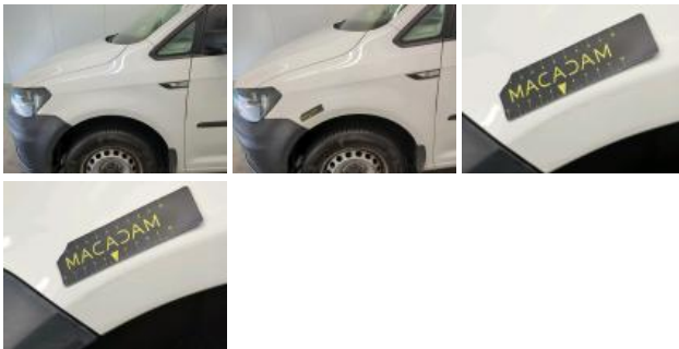
Outer sill L, Dent(s) and scratch(es), Repair and paint (complete)
