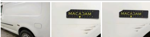
Wing RL, Scratch(es), Repair and paint (complete)
