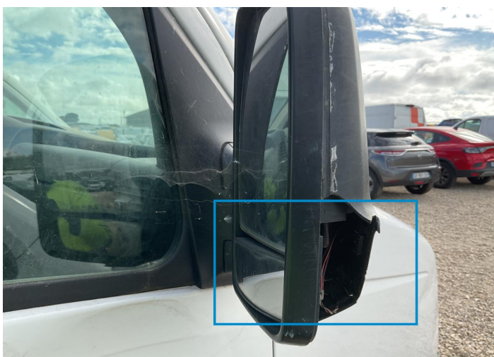
21. Mirror / Front Right Bodywork / Breakage / Hole -
