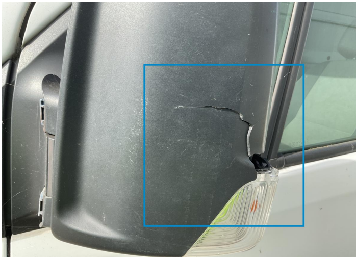
27. Mirror / Front Left Bodywork / Breakage / Hole -
