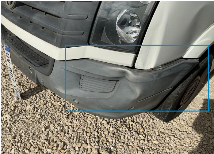
25. Bumper / Front Bodywork / Breakage / Hole -
