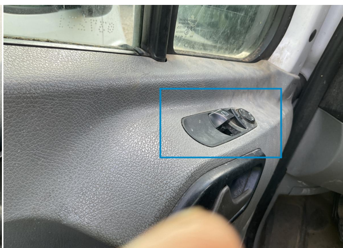
4. Window Switch / Front Left Interior / Broken -
