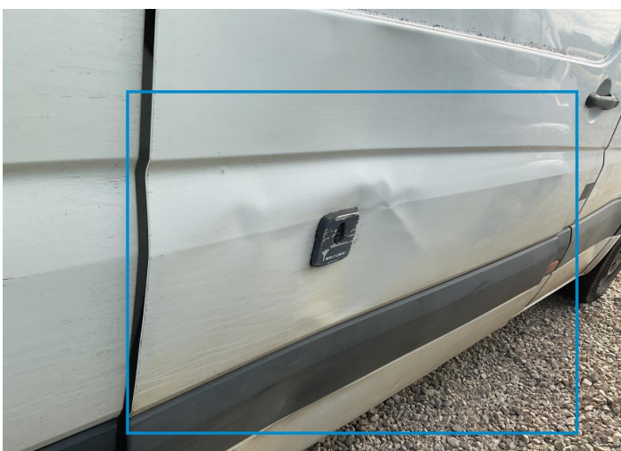
16. Door / Back Right Bodywork / Dent / Dent -
