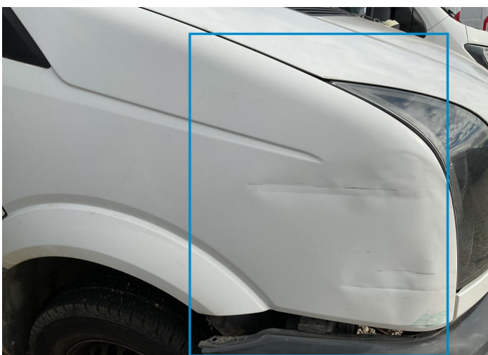
22. Fender / Front Right Bodywork / Dent / Dent -
