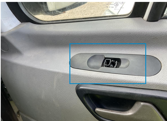
20. Window Switch / Front Right Interior / Broken -
