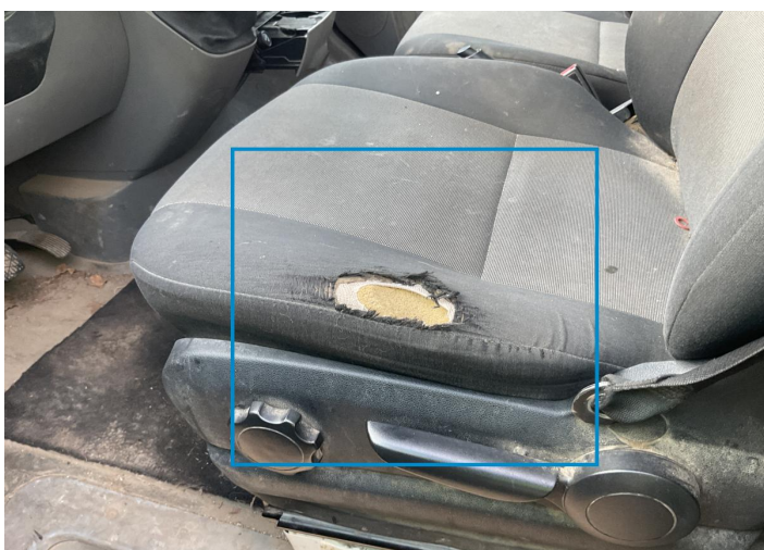
3. Seat / Front Left Interior / Ripped -
