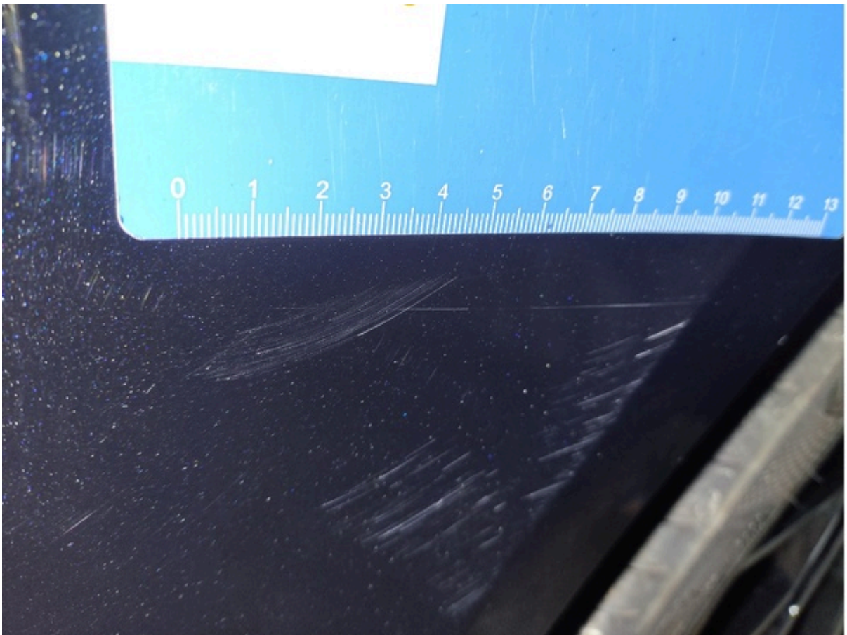
Bakdörr Spot repair Repor 2 000 kr
