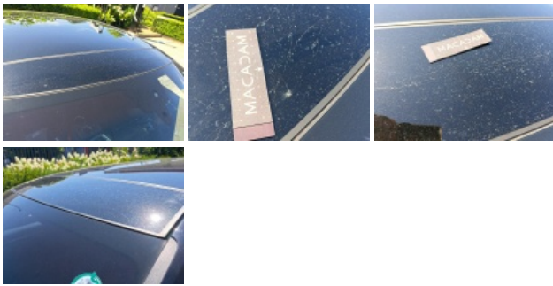
Panoramic roof, Broken, Replace
