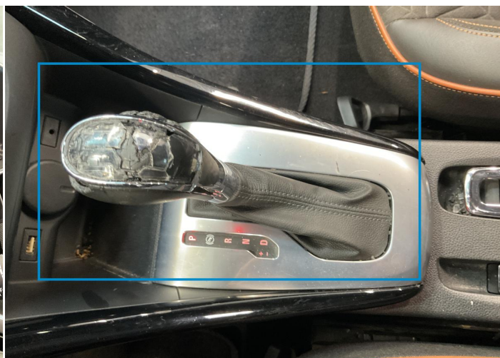
2. Gear Knob Interior / Broken -
