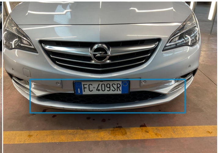
8. Shield Grid / Front Center Bodywork / Breakage -
