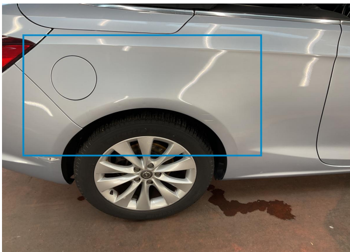
21. Fender / Back Right Bodywork / Dent -
