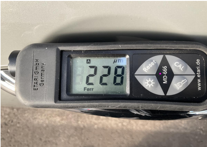
2. Door / Back Left Paint / Poor Previous Repair -
