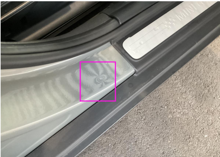
6. Rocker Panel / Center Right Bodywork / Dent / Dent -
