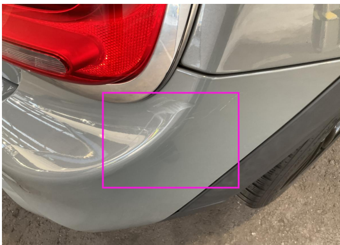
7. Corner Bumper / Back Right Bodywork / Dent / Dent -
