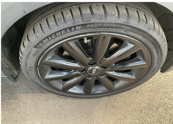
11. Rim / Front Right Out of Bodywork / Scratch -
