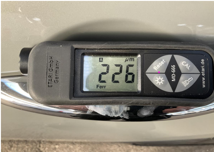
1. Fender / Back Left Paint / Poor Previous Repair -
