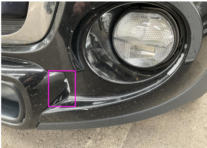
7. Bumper / Front Paint / Scratch / Scuff -
