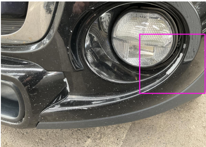
8. Bumper / Front Paint / Scratch / Scuff -
