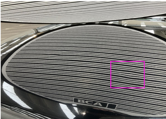
2. Roof Bodywork / Dent / Dent -
