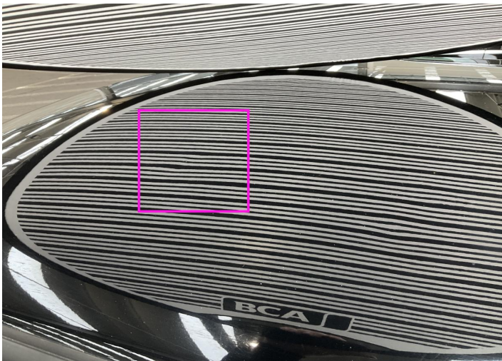
1. Roof Bodywork / Dent / Dent -
