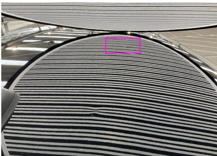
19. Roof Bodywork / Dent / Dent -
