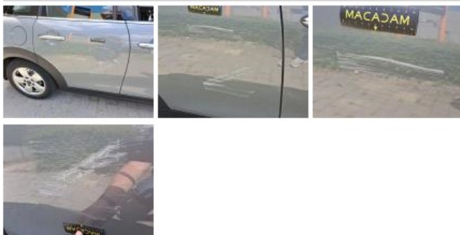
Door FR, Scratch(es), Repair and paint (complete)
