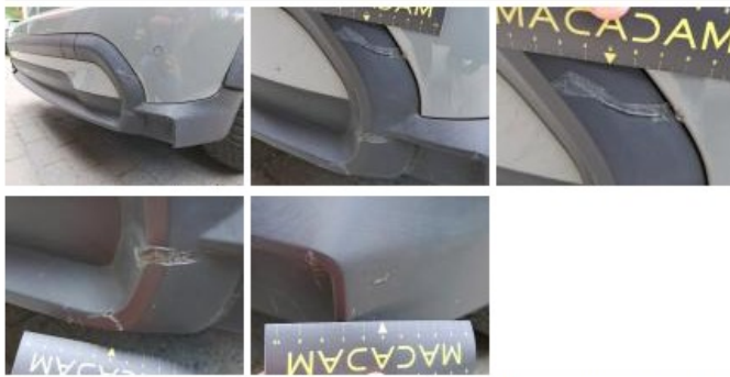
Wing trim RR, Deformed / Strained, Replace
