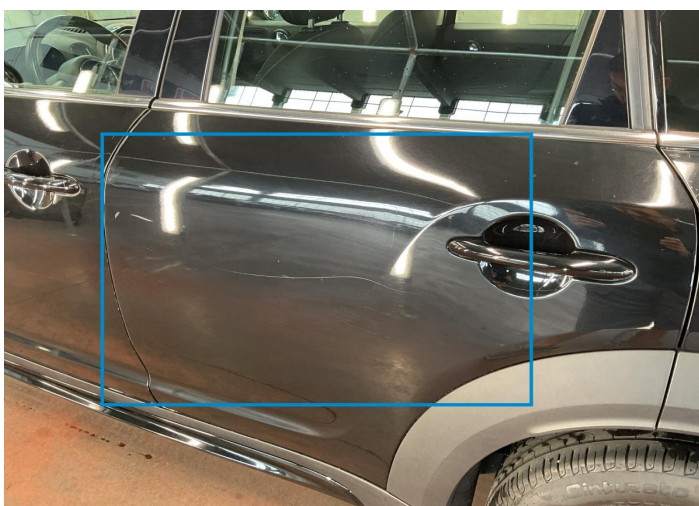
9. Door / Back Left Paint / Scratch / Line -
