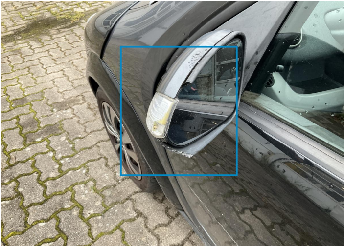
3. Mirror / Front Left Bodywork / Breakage / Crack -
