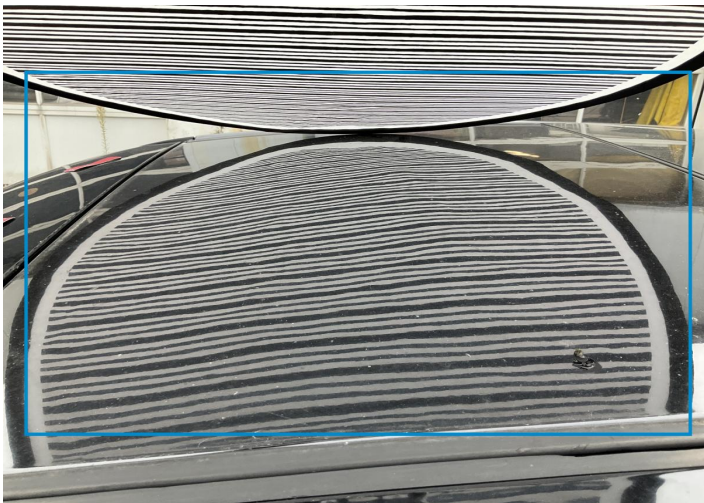
8. Roof Bodywork / Dent / Hail Area -
