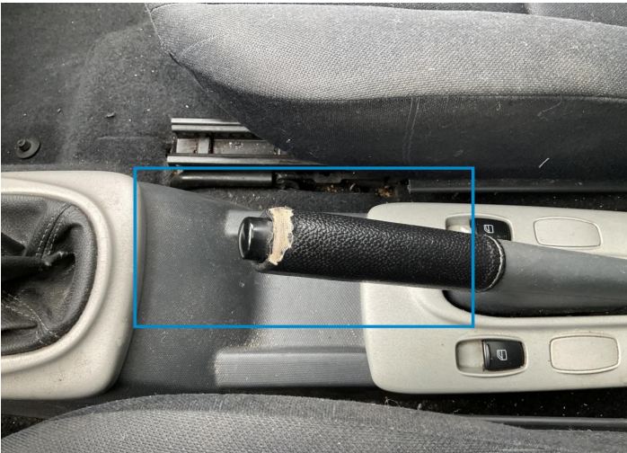
21. HandBrake Handle Interior / Ripped -
