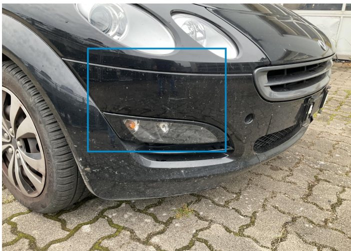
15. Bumper / Front Paint / Scratch / Scuff -
