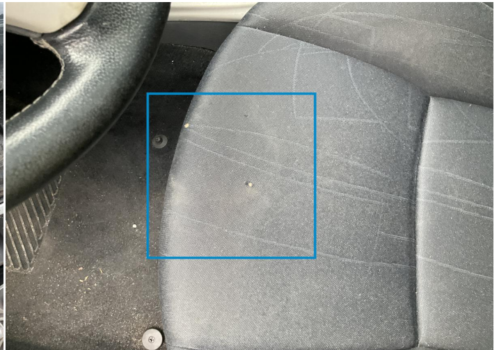
20. Seat / Front Left Interior / Holed -
