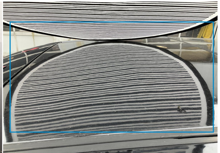
8. Roof Bodywork / Dent / Hail Area -
