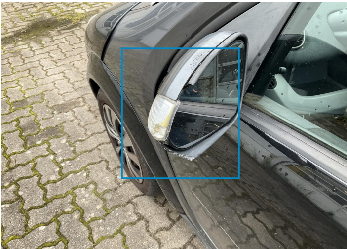
3. Mirror / Front Left Bodywork / Breakage / Crack -
