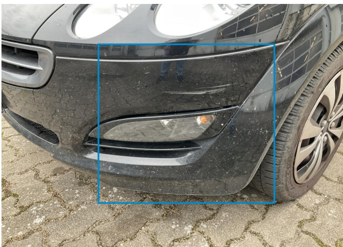
14. Bumper / Front Paint / Scratch / Scuff -
