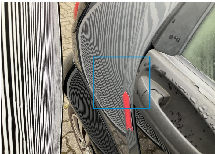
10. Side Panel / Back Right Bodywork / Dent / Dent -
