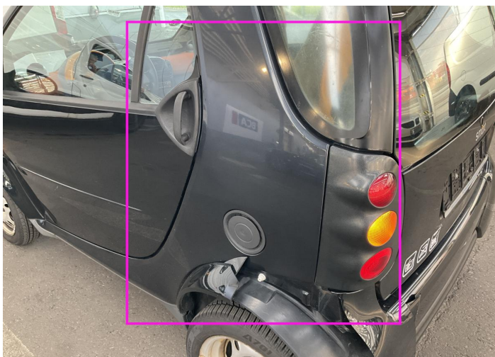
11. Side Panel / Back Left Bodywork / Dent / Dent -
