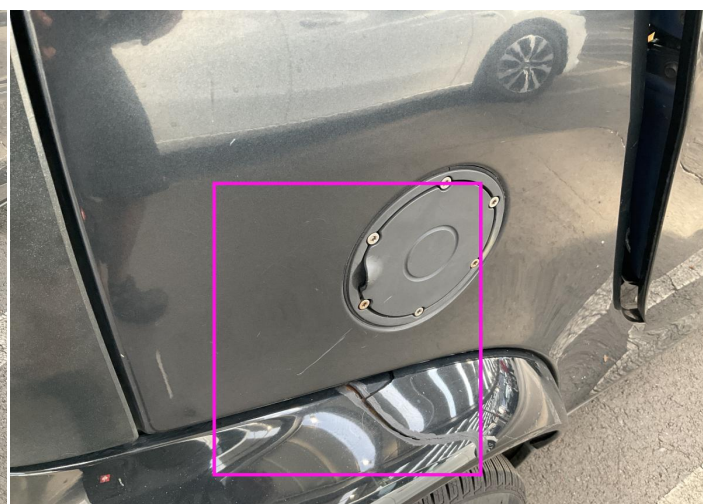
4. Side Panel / Back Right Paint / Scratch / Scuff -
