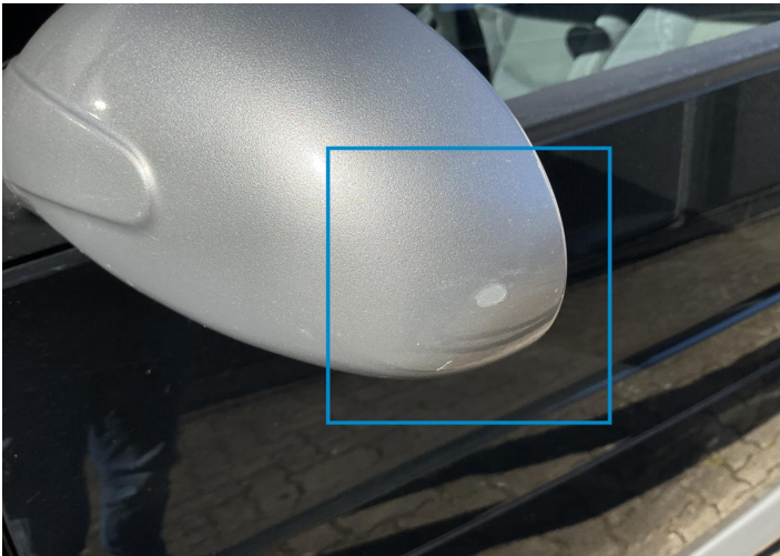
2. Mirror / Front Left Paint / Chipping -
