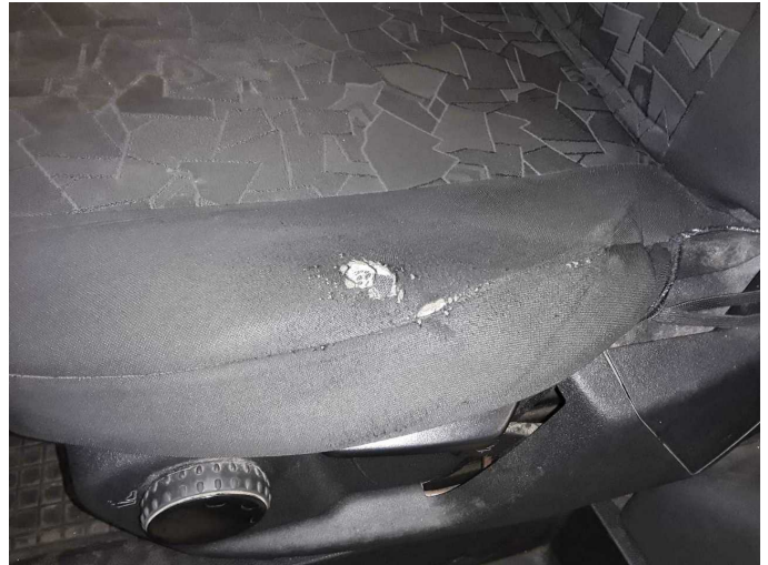
Damage 3: Seat - front: Protective Cover - left side - Broken / torn - Replace
