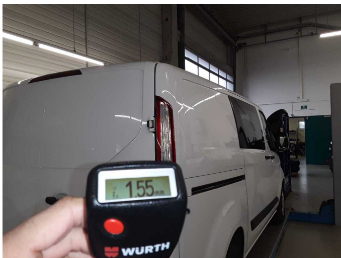
Side panel - rear right side: 1,550 µm
