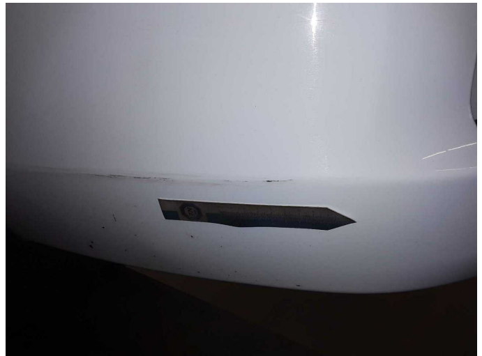
Damage 7: Rear bumper: Bumper - rear left side - Scratch(es) - Smart repair
