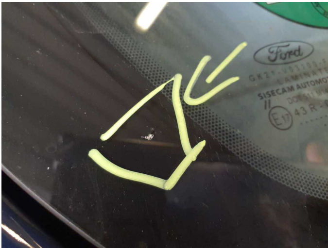
Damage 11: Vehicle glazing: Windscreen (Sichtbereich Rissbildung) - Stone chips - repair according to calculation
