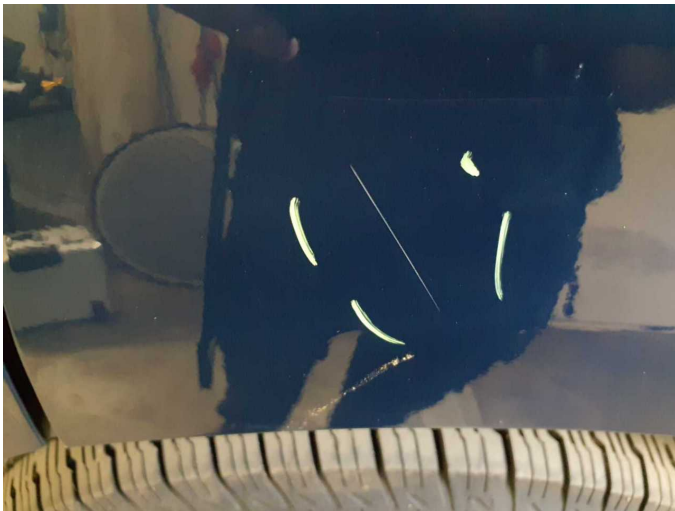
Damage 4: Mudguard - right side: Wheel arch - Scratched - Smart repair
