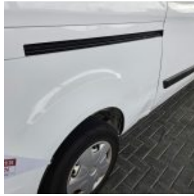
Damage Type Dent(s) & Scratch(es)
