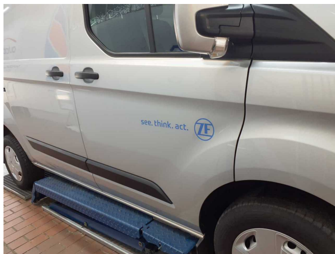
Damage 2: Body: Body - Glued / labelled - De-glue / neutralise
