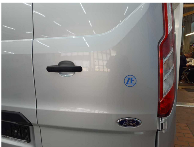
Damage 2: Body: Body - Glued / labelled - De-glue / neutralise
