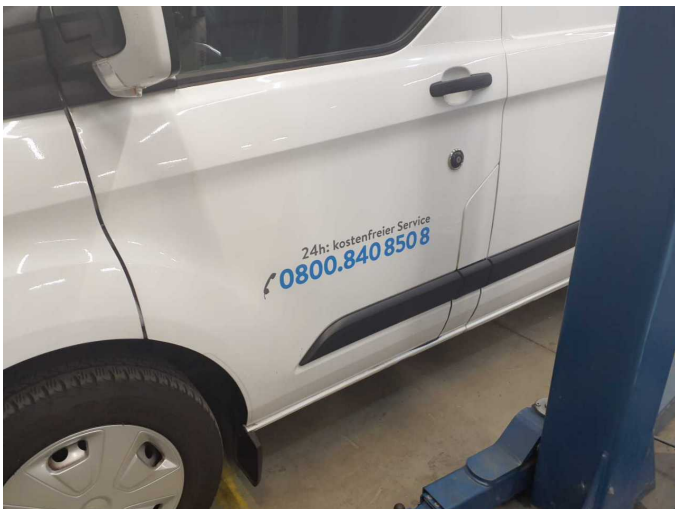
Damage 3: Body: Body - Glued / labelled - De-glue / neutralise
