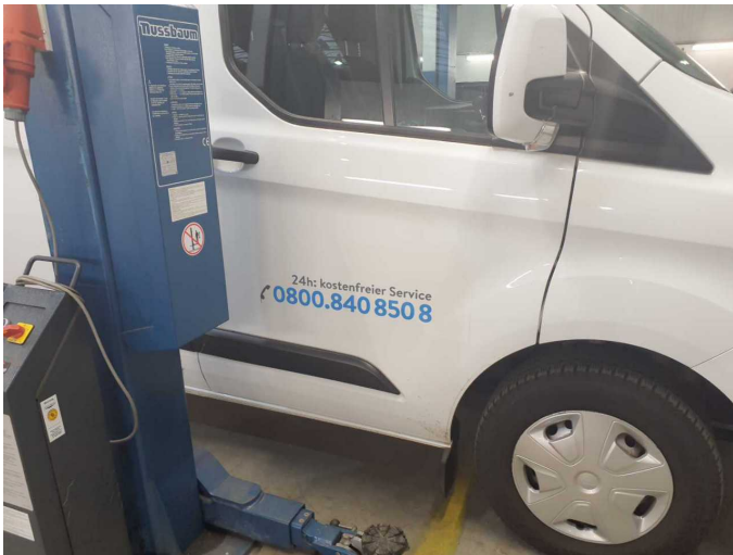
Damage 3: Body: Body - Glued / labelled - De-glue / neutralise
